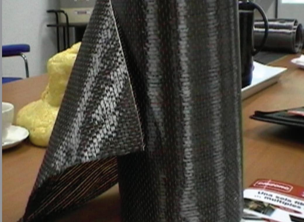
This technology is used to reinforce buildings made from concrete, masonry, steel or wood; it is also used for structural modifications and to improve their load capacity and safety level.
